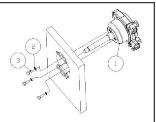
Fig 7. Installing ZTS Rotary Helm
