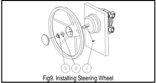
Turn steering wheel column until the keyway groove is top dead center. (This will help to keep the keyway from falling out during installation. Centering wheel adjustments will be made later while attaching cable end to tiller.)
