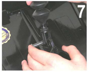
Attach the Actuator: Use the 5/16" snap & lock pins to attach the bottom of the actuator to the trim plate in Hole #3. NOTE: If needed, pressure adjustments can be made to suit your boat after a sea trial.
