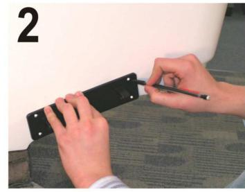
Mark Mounting Holes: Use the hinge as a template. Also make sure that you can mount the hinge in the same location on the other side of the boat.
