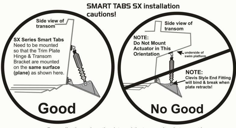
For applications where the plate and the transom bracket can not be mounted on the same surface (plane) use the Smart Tabs Stainless Steel Series, or call 800-233-0194 for advice!
