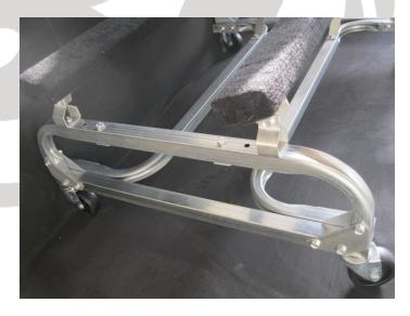
The brackets you see under the carpeted bunks can be positioned in two different locations depending on the width of ski's hull.
